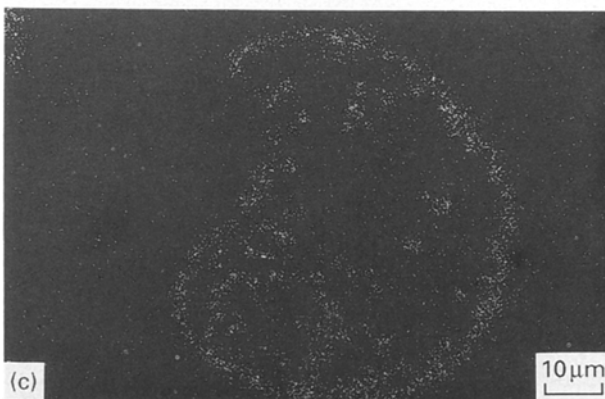
Figure 6 (a) Metallic iron grain containing TiC or Ti(O, C) produced at 1450 °C from minestone M, (b) elemental distribution map for Fe, (c) elemental distribution map for Ti.
