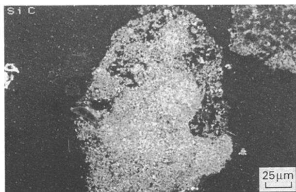
Figure 4 SiC particle obtained by reduction of minestone M at 1450 °C.
