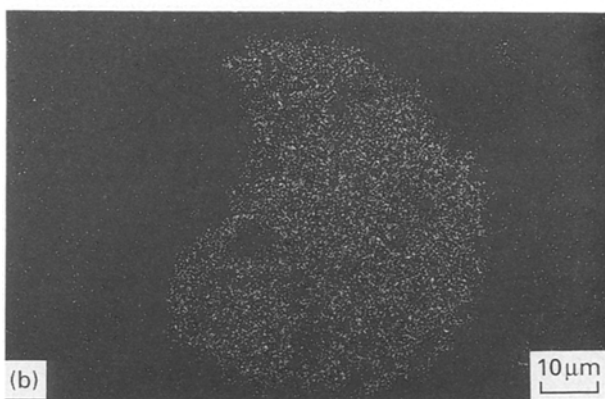
Figure 3 Particle obtained by reduction of minestone M at 1450 °C, showing SiC at the periphery and a core of Al 2 O 3 containing unreacted carbon.
